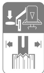
3. **17** Press and hold the operating handle left (12) and push the operating handle right (13) down to the half to split the log slowly first.
